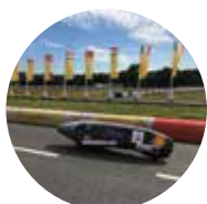
SHELL ECO-MARATHON VEHICLE In 2019 the vehicle fully developed by the students from the Technical University of Košice managed to drive 825 km using only 1 litre of fuel
